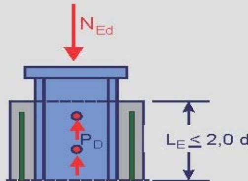
load introduction by headed studs within the load introduction length  $L_E$
