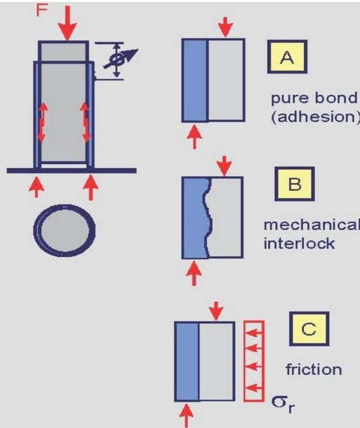
Outside the area of load introduction, longitudinal shear at the interface between concrete and steel should be verified where it is caused by transverse loads and / or end moments. Shear connectors should be provided, based on the distribution of the design value of longitudinal shear, where this exceeds the design shear strength  $\tau_{Rd}$ .
